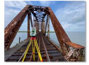
two programs that, when combined, provide a georeferenced and adjusted point-cloud (LAZ or LAS file). Once we had the LAS or LAZ file, we ran some quick checks with the help of a program called Global Mapper. The last step was data extraction. For this, we used TopoDOT, an application that works inside MicroStation that is used to import and extract 3D models from point clouds.
